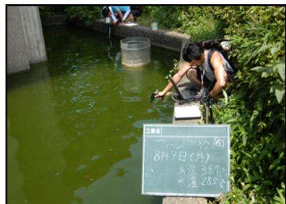
Plate 1 In-situ measurement of rich Chl-a content pond water using FieldSpec Pro Spectrometer derived specific hyper-spectral reflectance pattern at the VR and NIR region.
